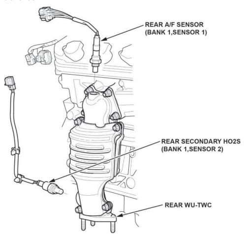
12. Remove the rear catalytic converter.
