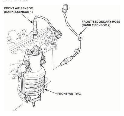
5. Remove the front catalytic converter.
