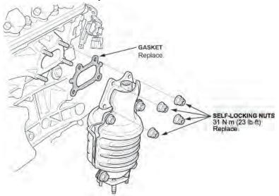
6. Install the new covers on the new front catalytic converter, then transfer the original A/F sensor and secondary HO2S sensor onto the new front catalytic converter.
