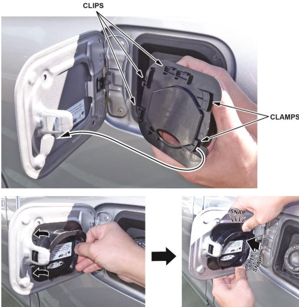
6. Make sure the fuel fill door closes and latches without contact or interference from the mis-fuel inhibit device and surrounding area.
