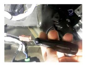
Special tool YRW5000070 to pop up the white retainer to release the connector shell. Note this can be done at the IPMB or at the camera itself.
