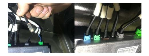
Camera lead shown with connector shell removed. Without the connector shells the leads can be swapped at the IPMB
