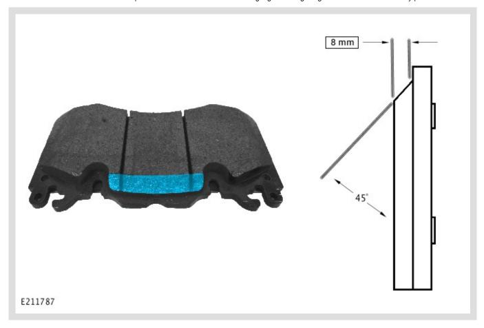
Use a suitable file to chamfer the new front brake pads as shown.
