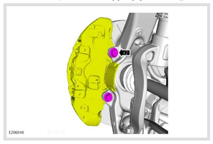
Install the brake caliper.
