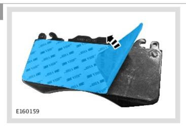
Gently remove the brake pad backing.
