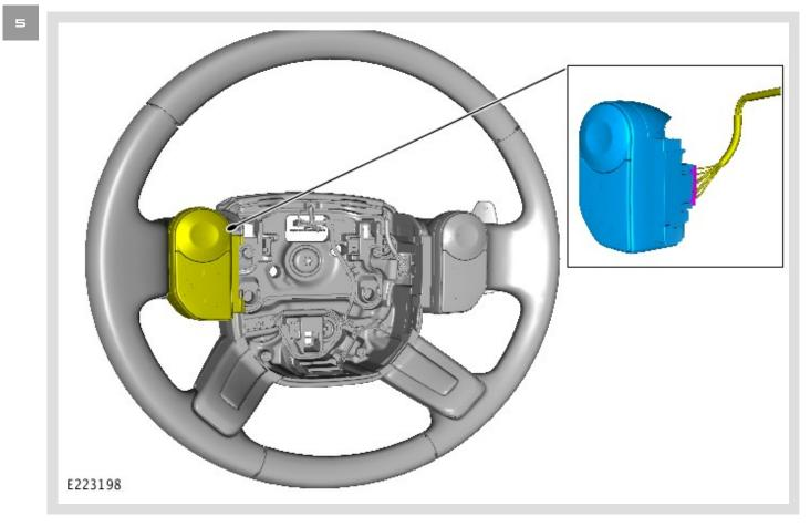
Remove and discard the steering wheel left control switch.
