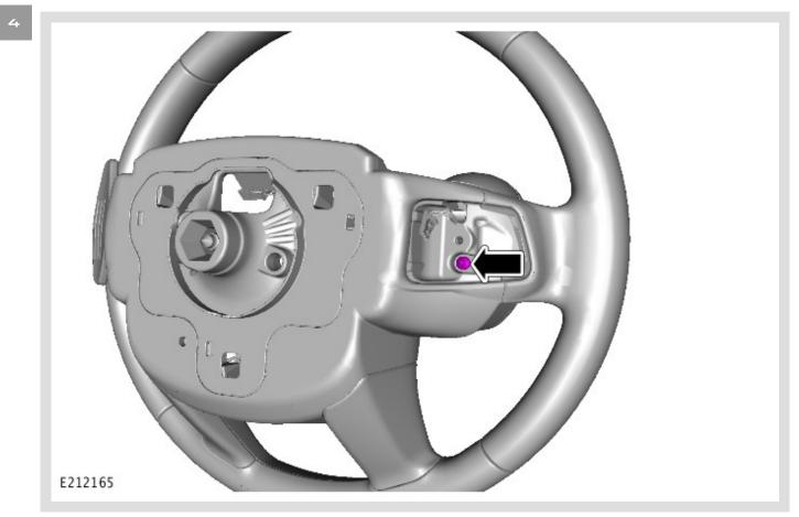
Remove the steering wheel left control switch fastener.
