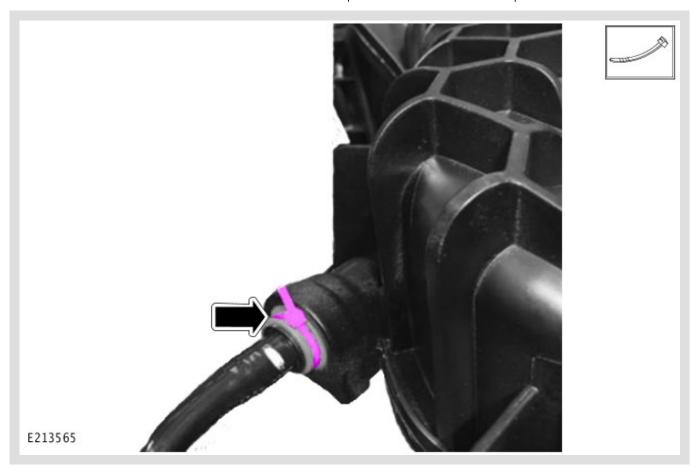
Install a cable tie around the locking ring.
