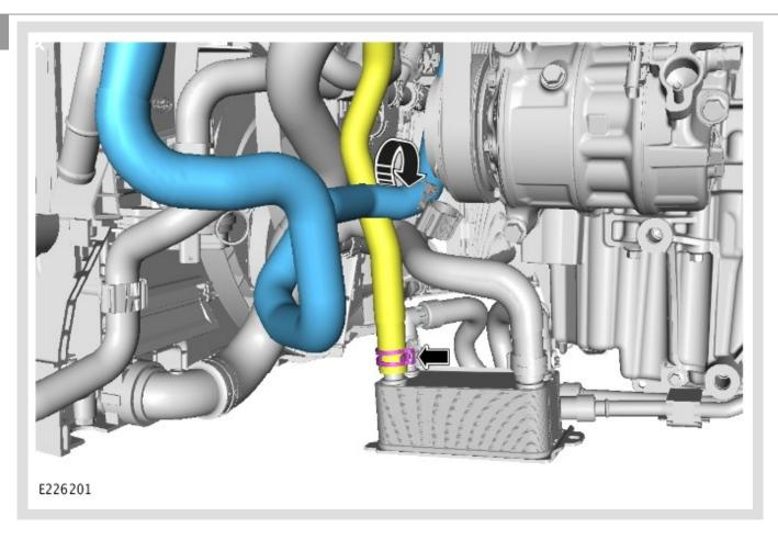
Remove the transmission oil cooler hose fastener and move the oil transmission cooler hose to the correct position.
