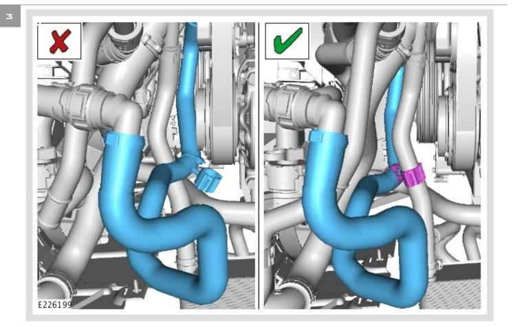
Inspect the engine coolant hose.
