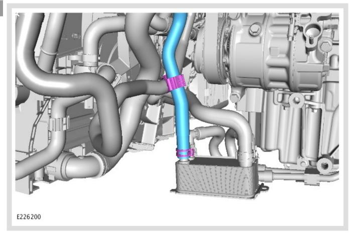
Install the transmission oil cooler hose in the correct position, making sure to secure the transmission oil cooler hose fastener.
