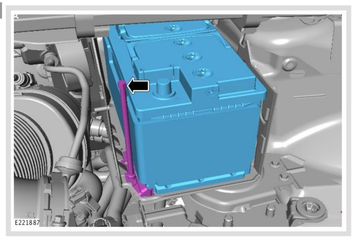
Remove the vehicle start up battery clamp.
