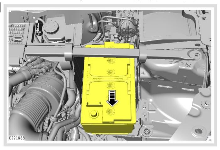
Move the vehicle start up battery forward.
