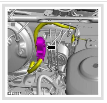
Disconnect the Anti-Lock Brake System (ABS) control module connector.
