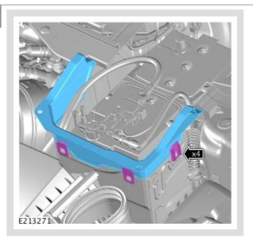
Remove the vehicle start up battery tray extension.
