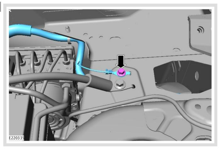
Remove the ground cable fastener.
