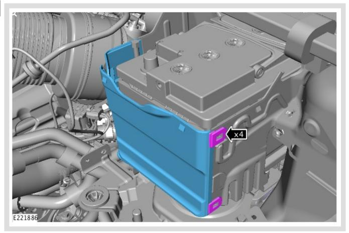
Remove the vehicle start up battery tray front panel.
