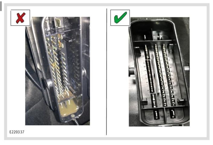
Visually inspect the ABS control module for water ingress.
