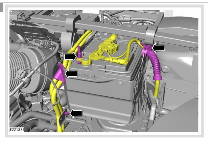
Remove the positive (+) battery cable mounting from the vehicle start up battery tray.
