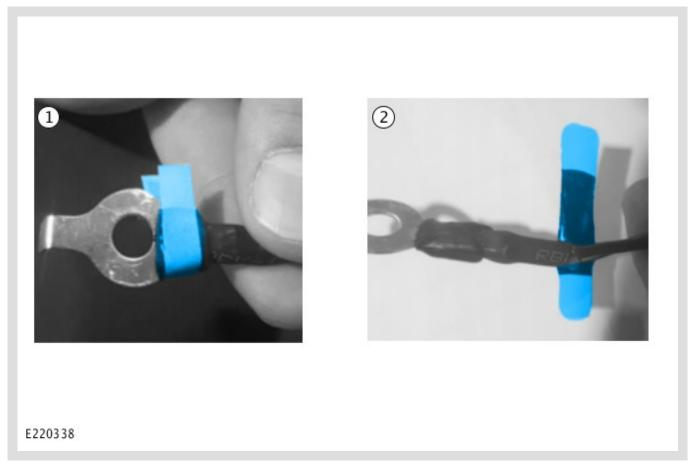
Install the butyl tape to the areas shown on the ground cable.
