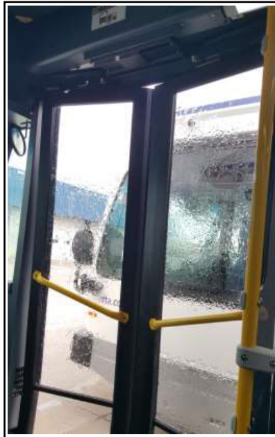
Figure 6 - Typical Location of Overhead Sensor Assembly mounted over Novabus Doorway
