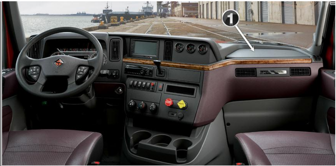
1. Fuse Panel Cover
