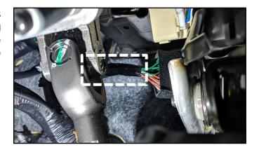
2a. If any individual wire(s) is damaged, (broken copper or split) then skip to the "Wire Repair Procedure" on page 4.
