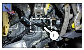
Refer to the procedure outlined on <u>TB023 Technician Basics</u> on KGIS to solder two (2) wires together using 60-40 rosin-core solder and repair damaged copper wires.
