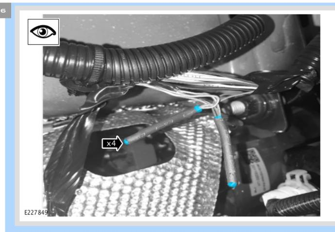
Visually inspect both sides of the heat shrink for 1-2 mm of glue to make sure the splice is fully sealed.
