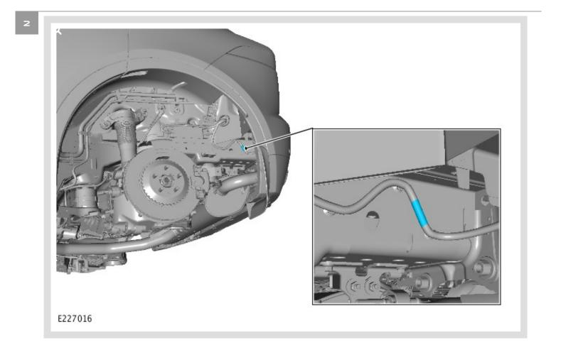
Unwrap the body wiring harness protection and access the body wiring harness located in the area shown.
