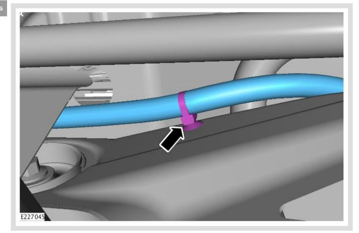
Install the rear axle wiring harness.
