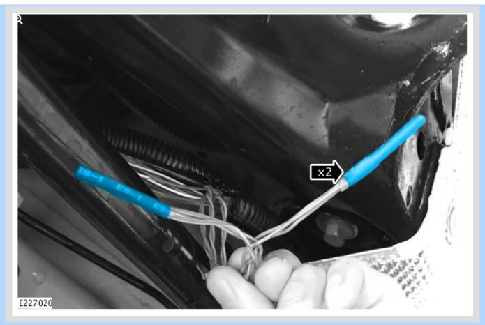
Apply glue lined heat shrink to splices as shown:
