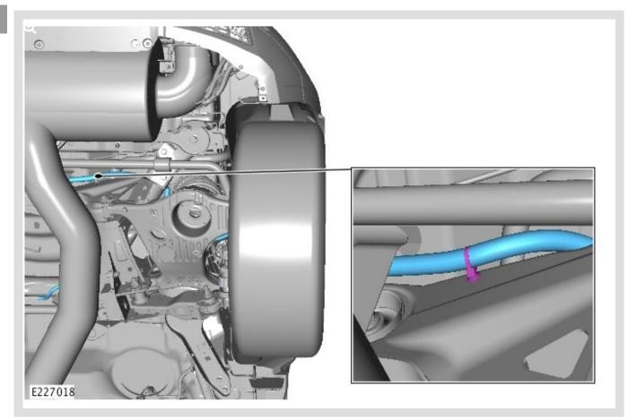
Locate the rear axle wiring harness.
