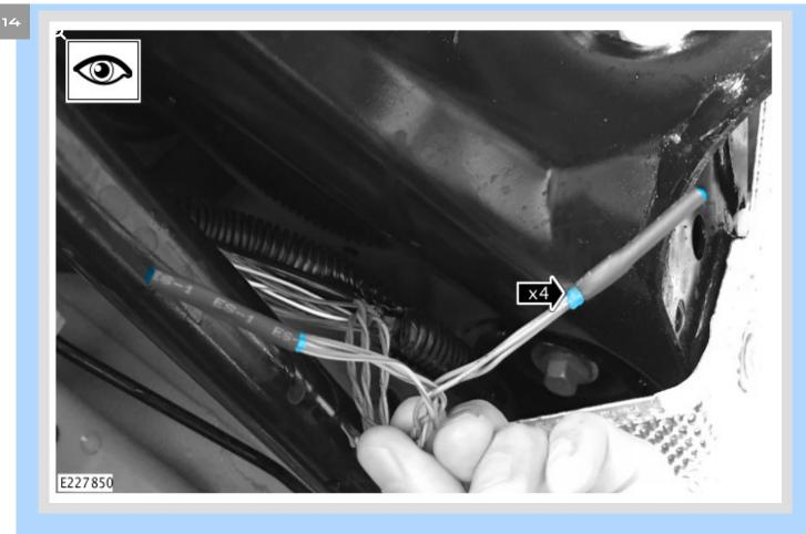
Visually inspect both sides of the heat shrink for 1-2 mm of glue to make sure the splice is fully sealed.
