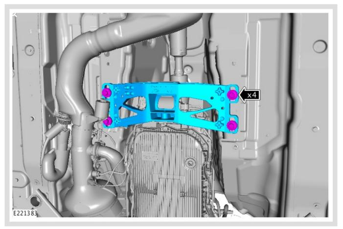
Loosen the 4 transmission mount fasteners.
