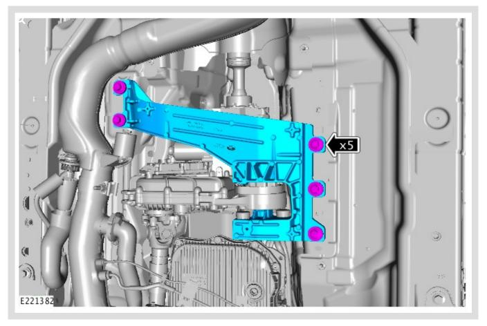
Loosen the 5 transmission mount fasteners.
