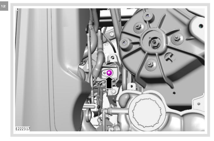
Tighten the left-side engine mount
