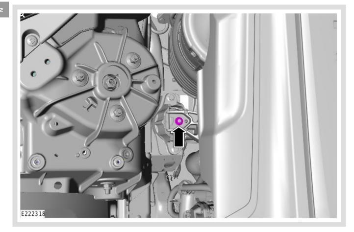
Loosen the right-side engine mount nut.
