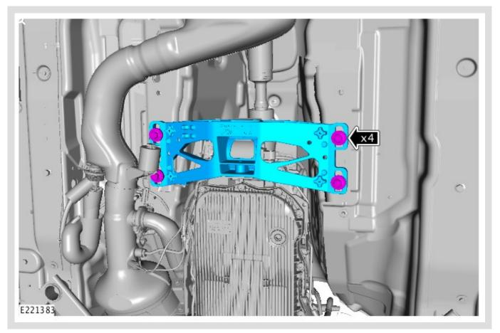
Tighten the transmission mount fasteners.
