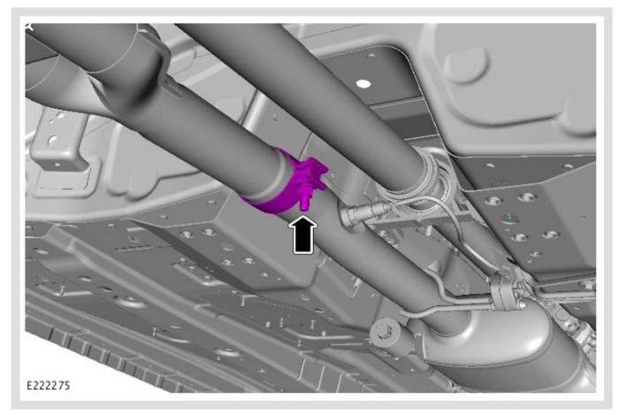
Tighten the exhaust clamp.
