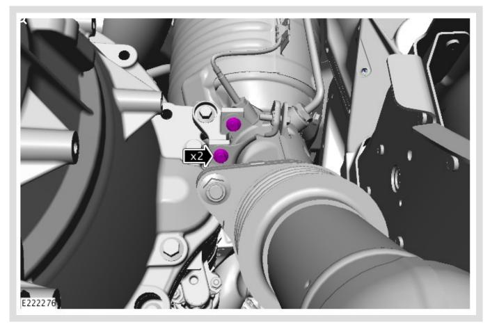
Tighten the 2 DPF fasteners.
