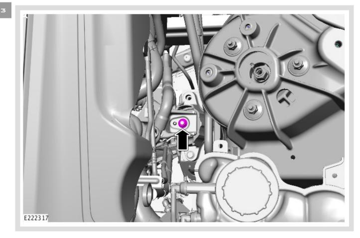
Loosen the left-side engine mount nut.
