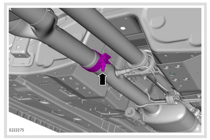
Loosen the exhaust clamp.
