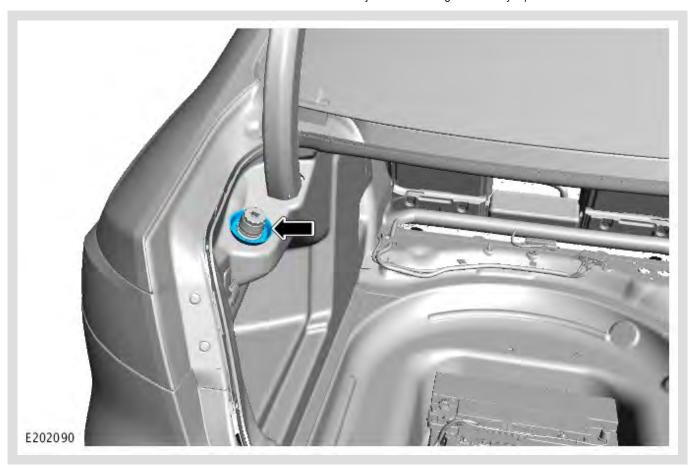
Remove the Diesel Exhaust Fluid (DEF) filler surround.
