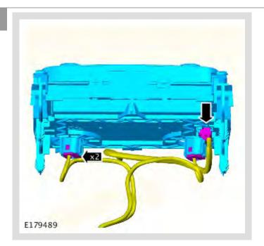
Disconnect the wiring harness from the rear seat climate control module.
