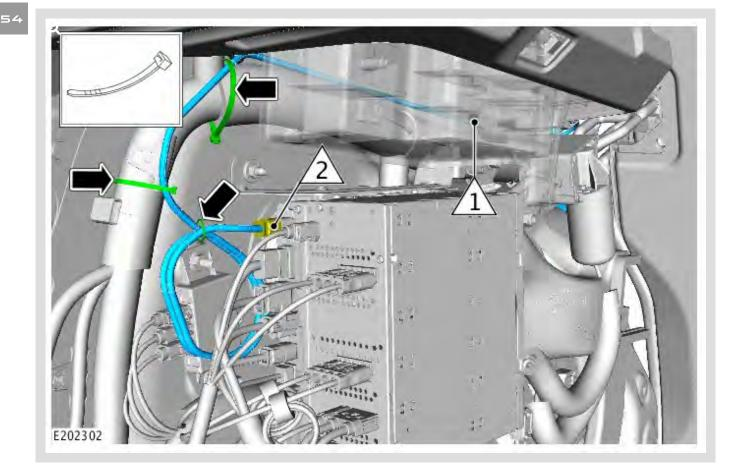
Install the same color connector on the new IMC rear link lead cable (**2**) to the Infotainment Master Controller (IMC).
