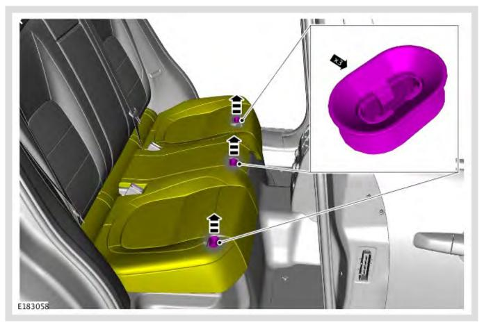
Release the rear seat cushion retaining clips.
