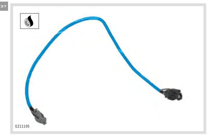
Apply felt anti-rattle tape around the length of the replacement USB link lead.
