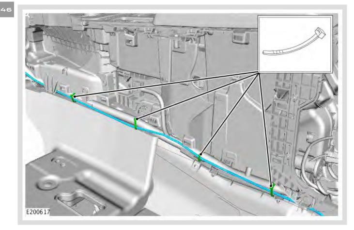
Route the new IMC rear link lead cable along the main harness below the floor console.
