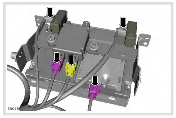
Remove the electrical connectors from the digital disc player, USB 2.0 hub, and Wi-Fi/Bluetooth™ antennas.
