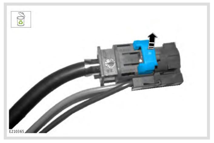
Using a suitable tool, remove and discard the locking tab from the electrical connector at each end of the original USB link lead.
