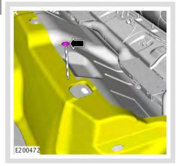
Remove the carpet retaining washer.
