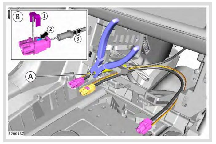
Making sure to **NOT** cut the 2 separate wires colored orange and brown, cut the main black section of the original IMC rear link lead cable (**A**).
