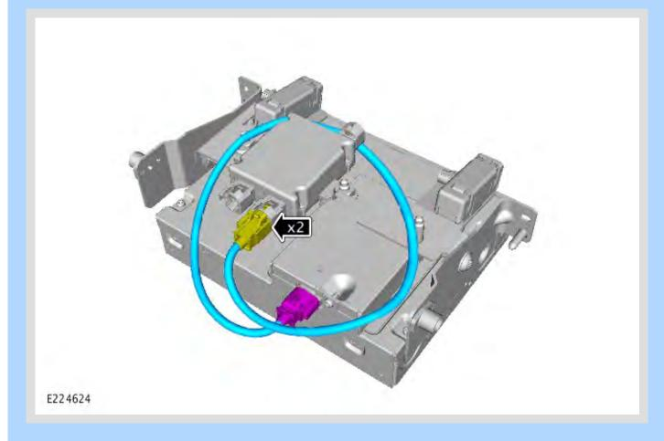
Install the electrical connectors to the digital disc player and USB 2.0 hub.
