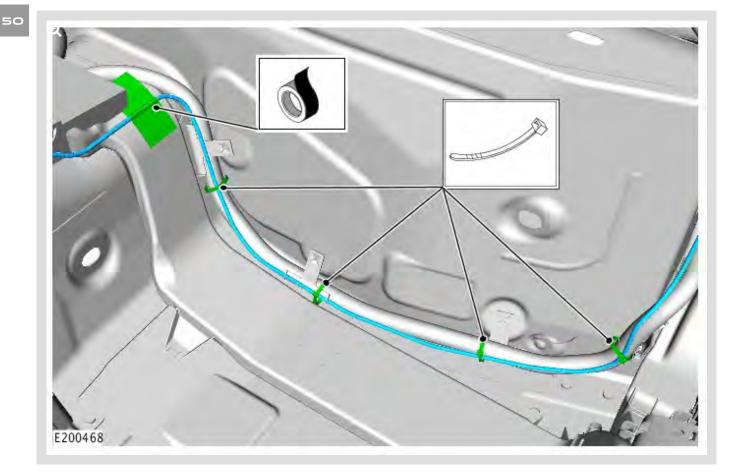
Route the new IMC rear link lead cable along the main harness in front of the rear seat base.
