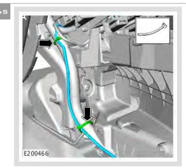
Route the new IMC rear link lead cable along the main harness towards the instrument panel.
