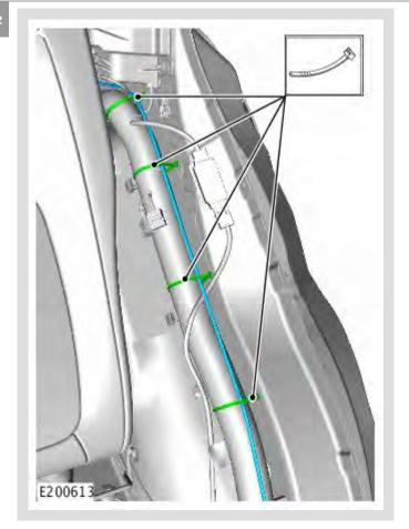
Route the new IMC rear link lead cable along the main harness above the wheel arch.
