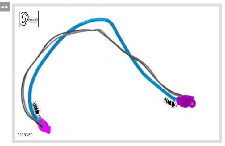
Install the replacement black coaxial USB link lead into the original electrical connectors.
