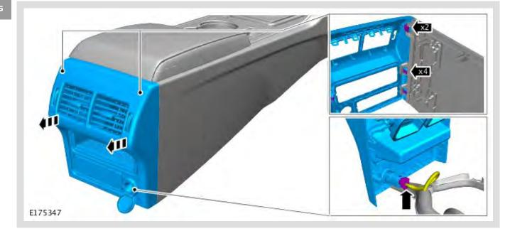
Remove the rear heater control panel.
