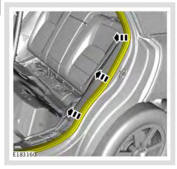
Reposition the rear left door aperture seal.
