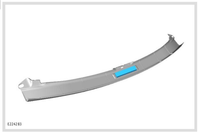
Install the double-sided self-adhesive foam to the luggage compartment header panel trim.
