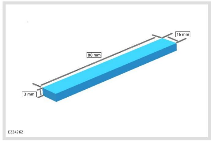
Measure and cut a suitable piece of double-sided self-adhesive foam to the dimensions shown.
