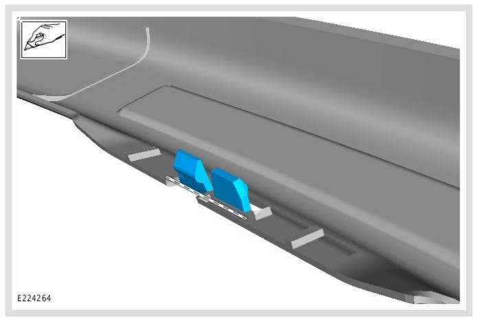
Use a suitable tool to cut the retaining clips from the luggage compartment header panel trim.
