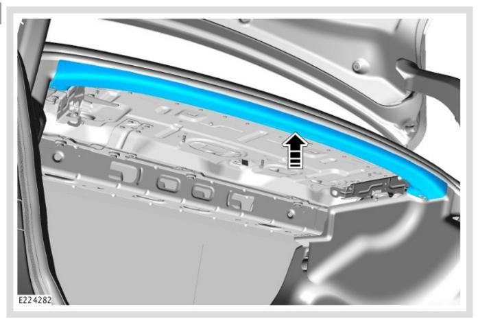
Apply firm pressure to the center of the luggage compartment header panel trim to make sure the self-adhesive foam has bonded.
