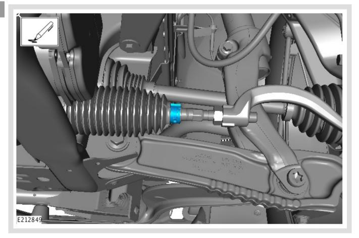
Apply yellow paint mark to the tie-rod bellow clamp to indicate completion of the repair.
