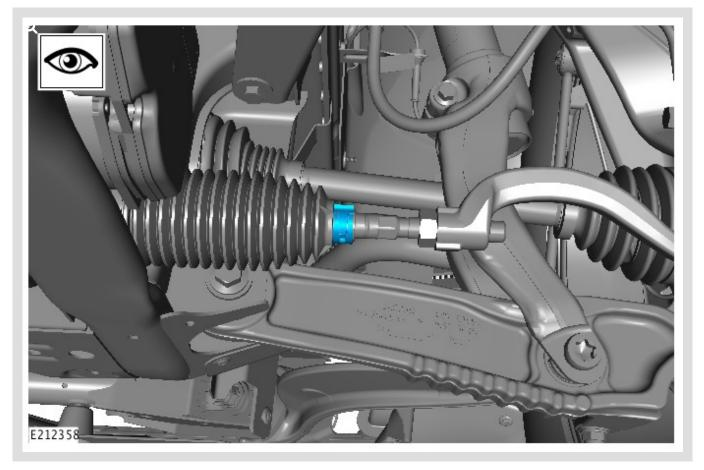
Inspect the tie-rod bellow clamp for a yellow paint mark indicating that the repair has previously been completed.
