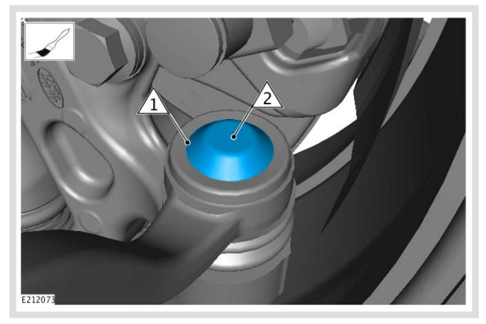
Apply the sealing wax to the tie-rod end retaining cap.
