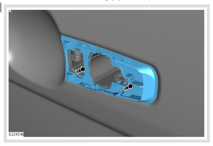
install the new front left door exterior handle gasket.
