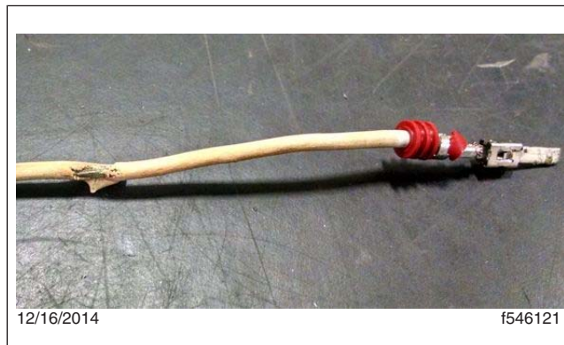
Fig. 2, Insulation Discoloration, Major
