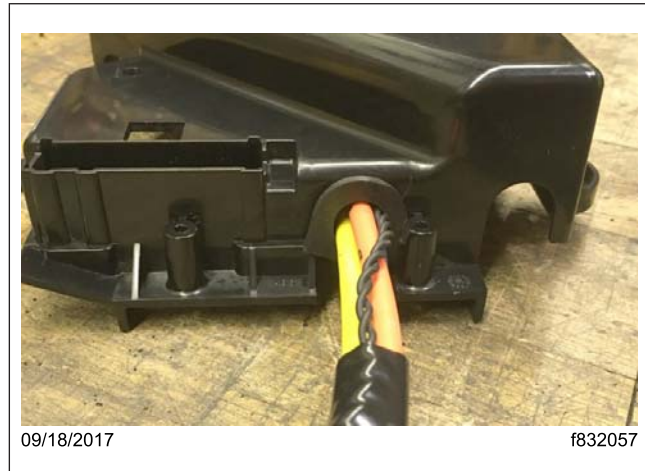
Fig. 6, Harness Routed through the New Opening
