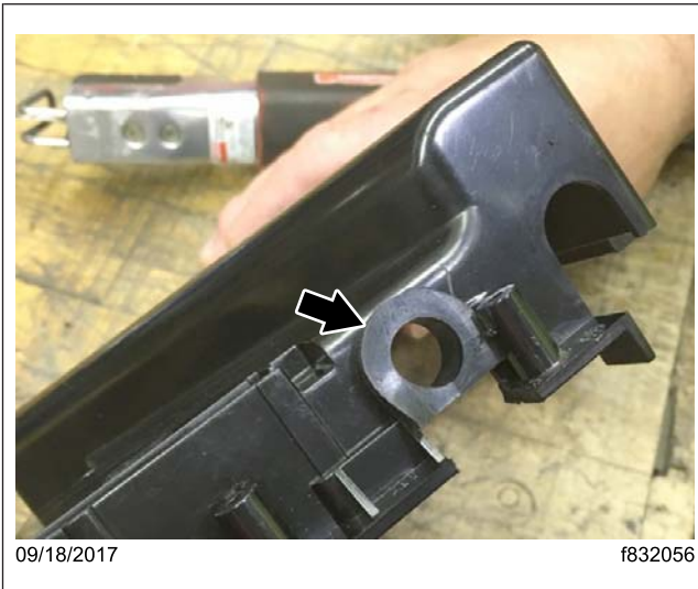
Fig. 5, Grommet Installed in the New Opening
