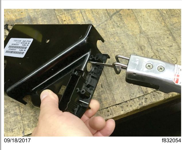
Fig. 3, Cutting the Slot for the New Opening
