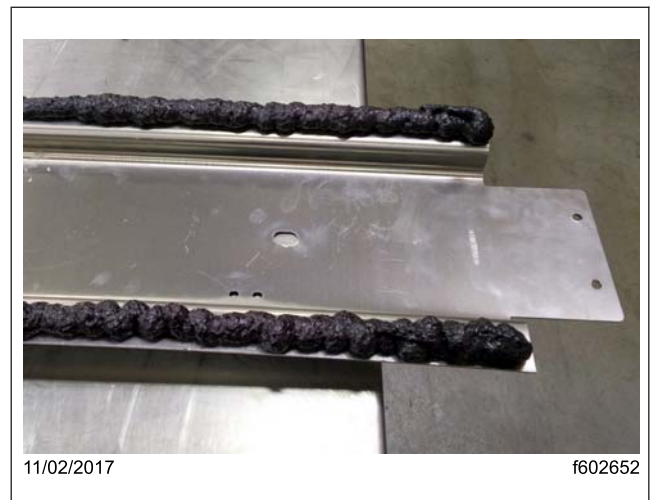
Fig. 5, Foam Sealant Applied on Roof Bow
