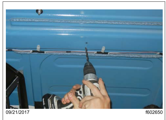
Fig. 3, Drilling the Holes for the Rivets
