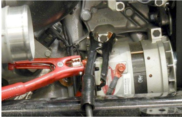
Fig. 7, For EPA10 and EPA04 engines, the starter path can be checked by loading the circuit at the alternator.
