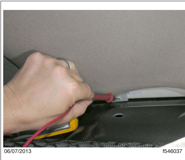
Fig. 5, Measuring the Resistance on the Thin-Film Antenna Lower Rivet
