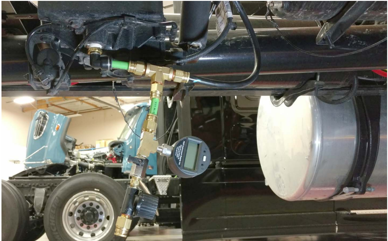
Fig. 4, Gauge Installation Using a Jumper Line with a Tee Fitting
