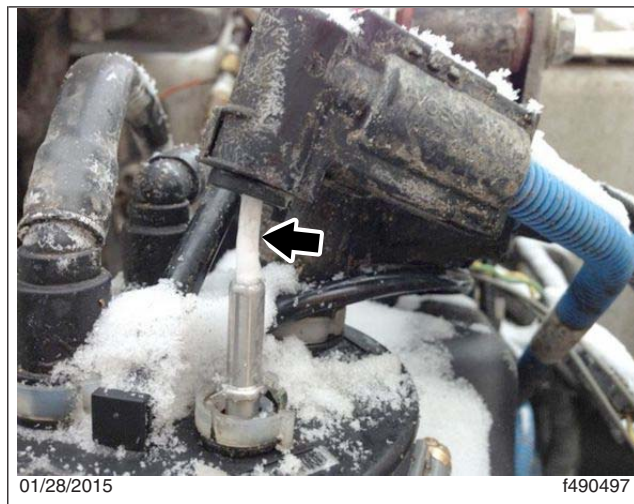
Fig. 1, Ice Expansion at the DEF Line Fitting
