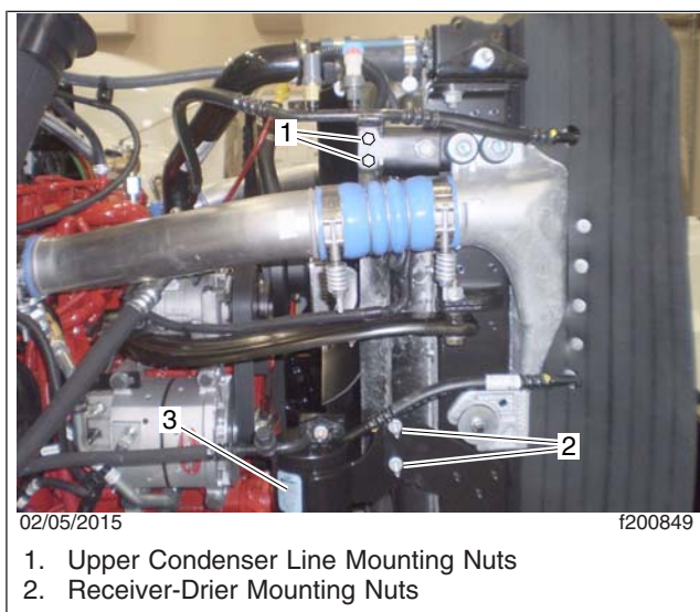
Fig. 2, Receiver-Drier Installation (typical)
