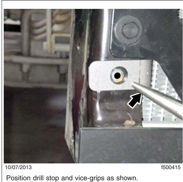
Fig. 4, Drill Stop Installation
