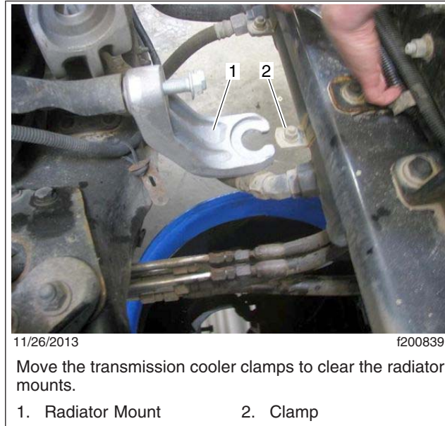
Fig. 3, Moving the Transmission Cooler Clamp
