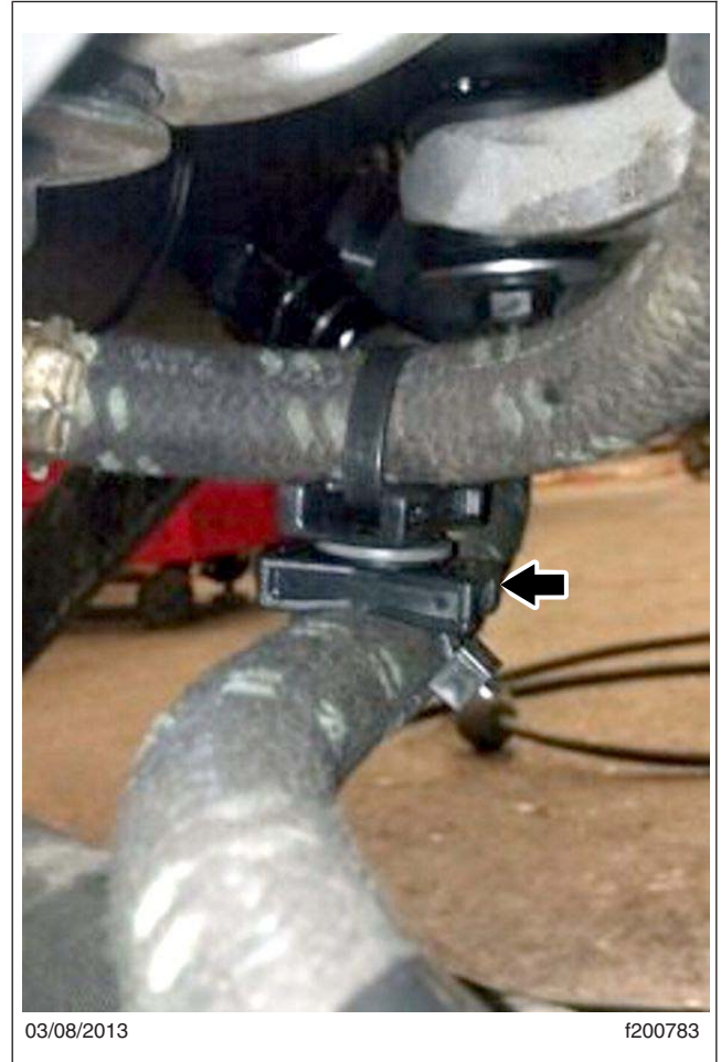
Fig. 20, Ziptie Swivel Installation
