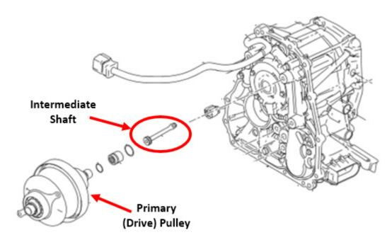
**VERY IMPORTANT:** In the unlikely event DTC P0A78 **AND** P1C2A are detected and set at the same time, follow the diagnostic procedures for BOTH DTCs to determine the fault **BEFORE** proceeding with reprogramming the ECM. In this case, the following 4 components must be replaced together **as a set** following the procedures supplied in the applicable Service Manual.
