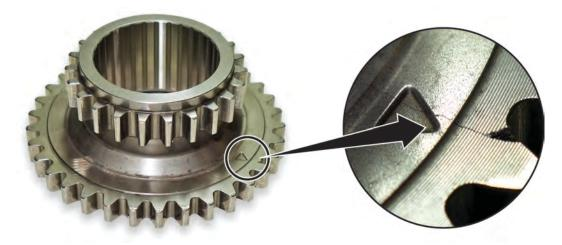
If the sprocket has hairline fractures, replace it along with the cam chain and any other affected parts.
