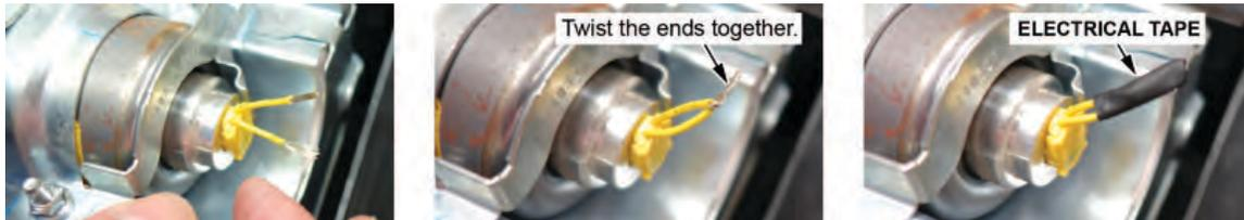
3.6. Tape the twisted ends with electrical tape.
