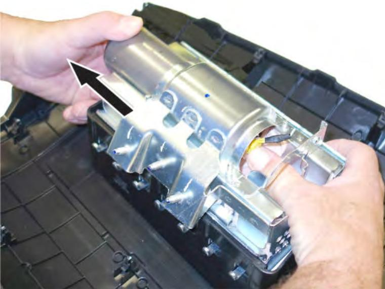
6. Put the original inflator into the new inflator box acquired from XPO. Make sure there is no other hardware in the box because if the package rattles, it will not be accepted by the courier.
