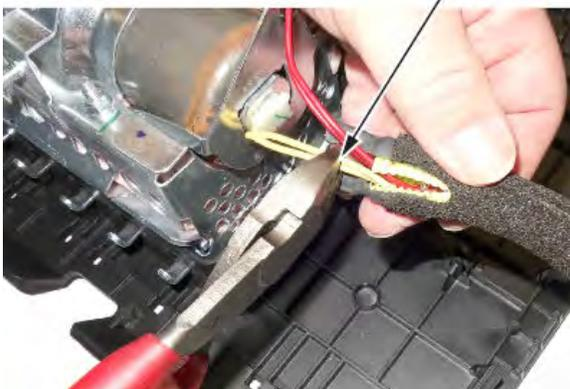
3.5. Strip away about 1 inch of the yellow wire insulation, then twist the wires together.
