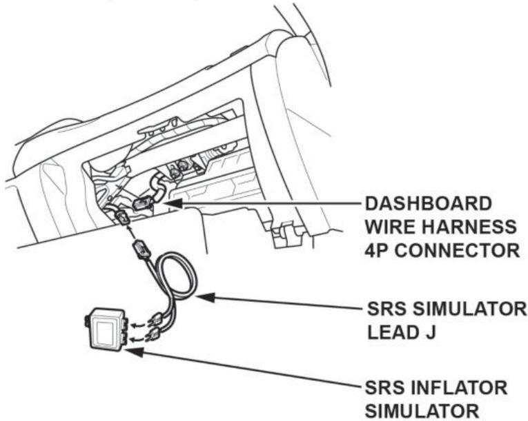
12. Connect the terminals of SRS simulator lead J to the SRS inflator simulator (2 Ω connectors), then connect SRS simulator lead J to the 4P connector as shown.
