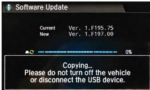
13. After the software update is complete, remove the USB update device and press **Continue**.
