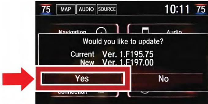
12. After the system reboots, the software update will start automatically. After the update has started, the installation is automatic and the technician does not need to stay with the vehicle.
