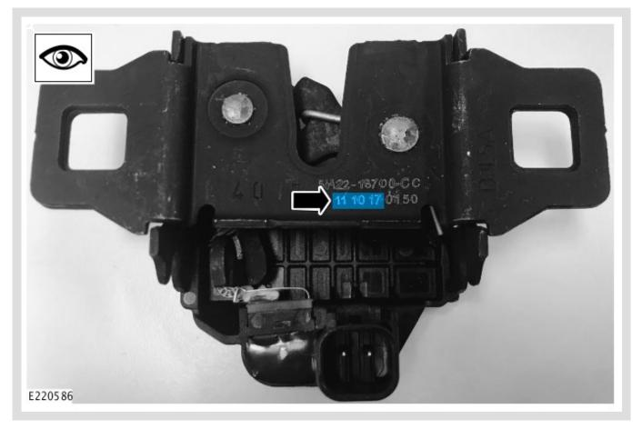
The date code (DD/MM/YY) of the new hood latch must be **23/11/2017 (23 November 2017)** or later.
