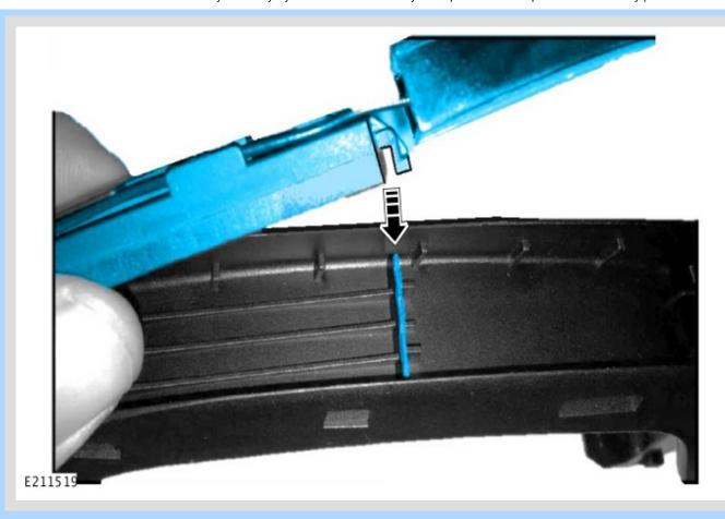
Install the antenna and electronic unit into the handle strap inner; align the clip with the handle strap inner rib.
