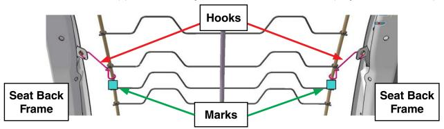
• If the paper wrapping on either of the vertical "anchor cords" has been chaffed through by any of the hook(s), re-wrap the affected area(s) with electrical tape before installing the new hook(s).
