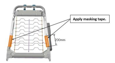
• Mark the locations (4) of the currently installed hooks for reference (only 2 are shown here).
