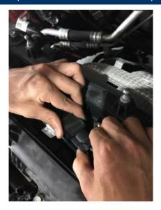
Remove the bolt from each of the 4 ignition coils using a 10mm socket with a 3/8" ratchet 3. and extension.
