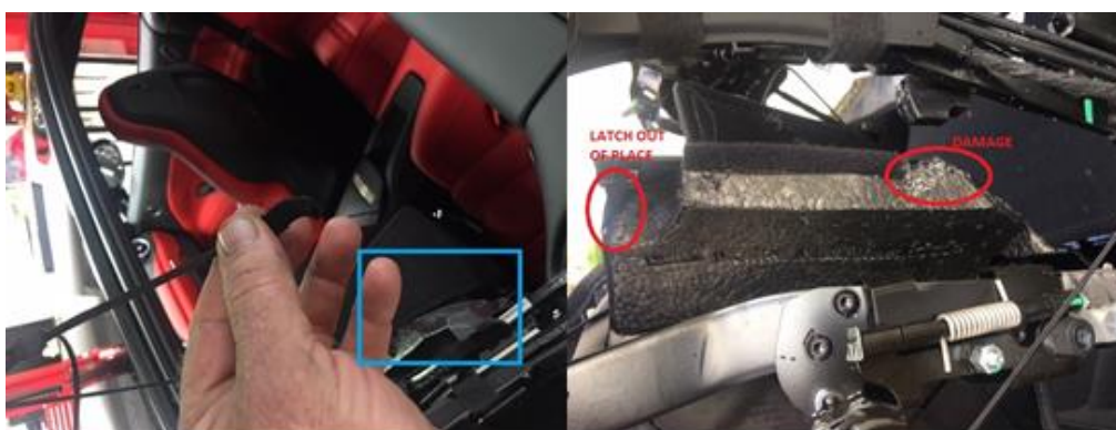
Figure 2 : Polystyrene location and damage
