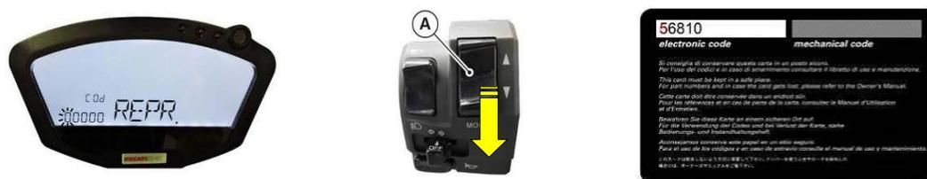
4) To confirm the entered digit, push **button (A)** up "▲" and enter the second digit of the code indicated on the Code Card.
