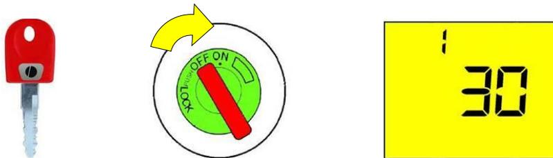
3) Perform a Key-OFF before the countdown of 30 tenths of a second displayed on the instrument panel is over and then remove the key.
