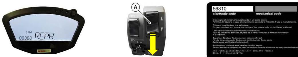
3) The first digit on the left starts flashing and it is therefore possible to enter the first digit of the code indicated on the Code Card by pushing **button (A)** down "▼" (the counter increases its value by one unit every time the button is pushed down "▼" until digit 9; then, it starts the sequence again).
