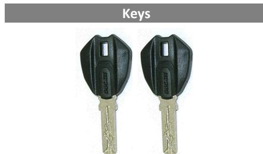
The **keys** are provided with passive transponder powered by the antenna integrated in the E-Lock control unit.
