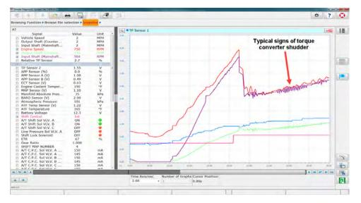
In a vehicle with a known good torque converter, Engine Speed, Input Shaft and Output Shaft speeds will all be smooth. See the example below:
