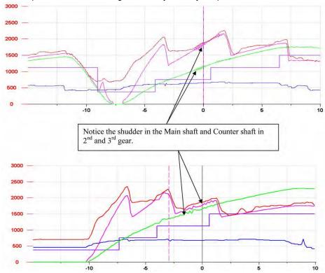
If you're feeling the vibration while under a steady cruise, look for Engine Speed to be briefly jumping above Main Shaft speed. This would indicate that the torque converter is experiencing a stick/slip condition as shown below:
