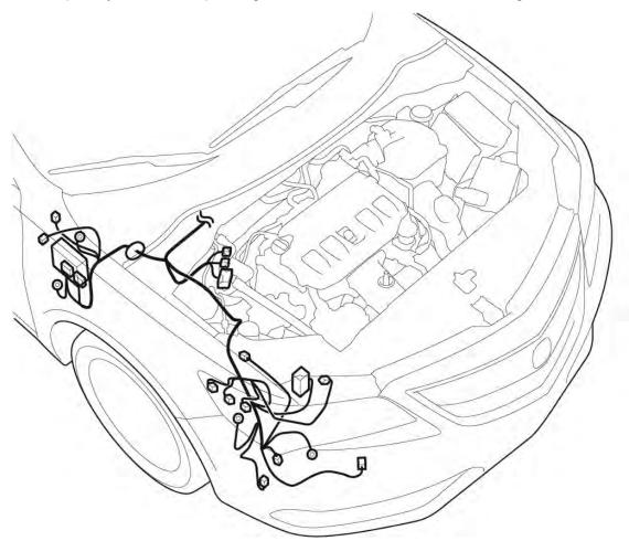
6. Starting at the interior of the driver's side, remove the harness. Follow the harness into the engine compartment.
