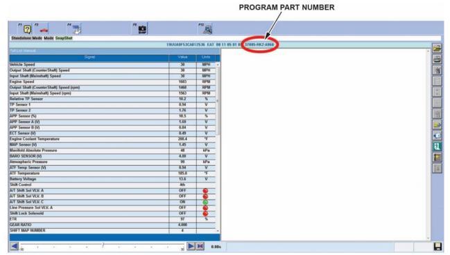
• If the program P/N is listed below (or later), the vehicle has been updated. Go to Service Bulletin 17-042, 2013–14 Crosstour V6: Judder from the Torque Converter Lock-Up Clutch After Software Update.
