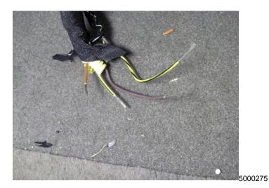
9. Remove 13 mm (1/2 in) of insulation from the seat and body harness wire ends.
