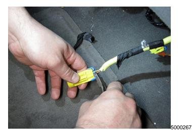
8. Cut off the two connector halves as close to the connector as possible.
