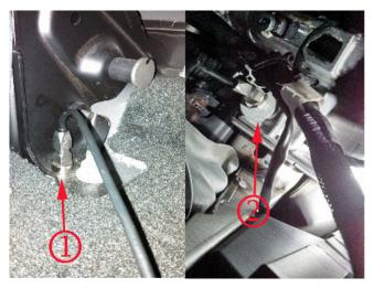
3. Using a Pico Oscilloscope Diagnostic Kit, mount the PicoScope vibration sensor on one of the two locations shown above.
