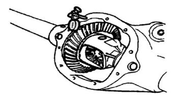
Install the J-25025 pins and the J-8001 indicator to the axle housing.
