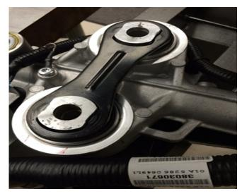
For vehicles with T1 vibrations under 20-25m/g's, replace steering bushing per parts catalogue. Utilize SI procedure "Steering Gear Mount Bushing Replacement" for replacement of the steering bushings.
