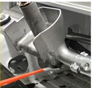
While pressing down on the passenger side pivot shaft, spray AC Delco Super Lube P/N 12346241 – US (P/N 10953474 – Canada) on the base of the pivot shaft assembly.
