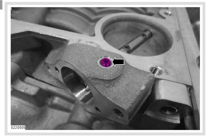
Remove the bypass valve set screw.
