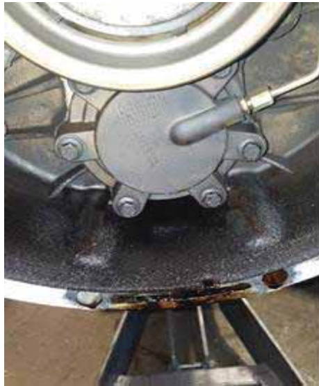
Engine Oil Accumulation in Bottom of Flywheel Housing
