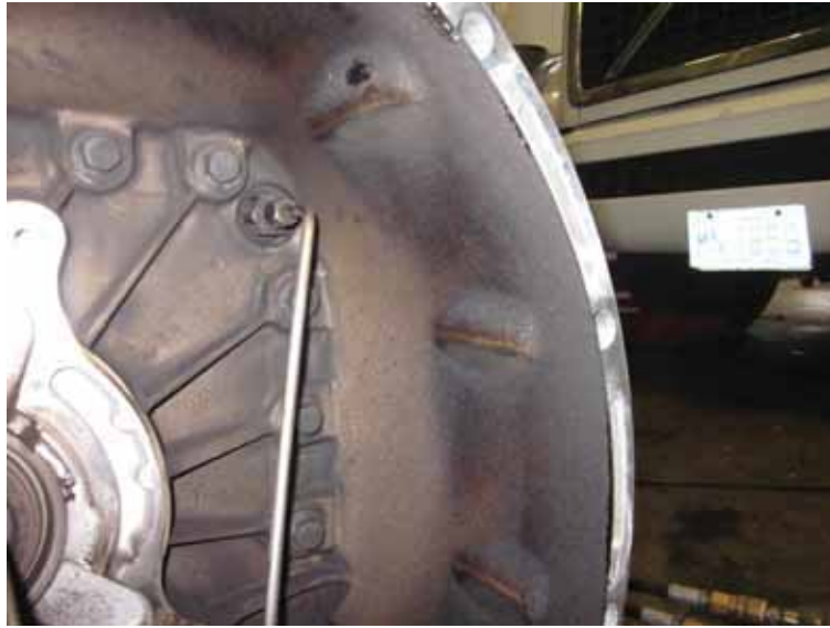
Oil Film visible on inner circumference of the Clutch Housing
