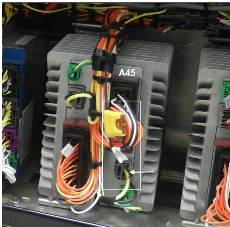
A45 MODULE & ELD GATEWAY MODULE CONNECTION
