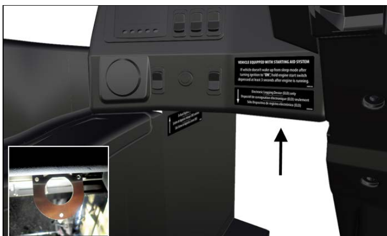
BRACKET POSITION UNDER DASH
