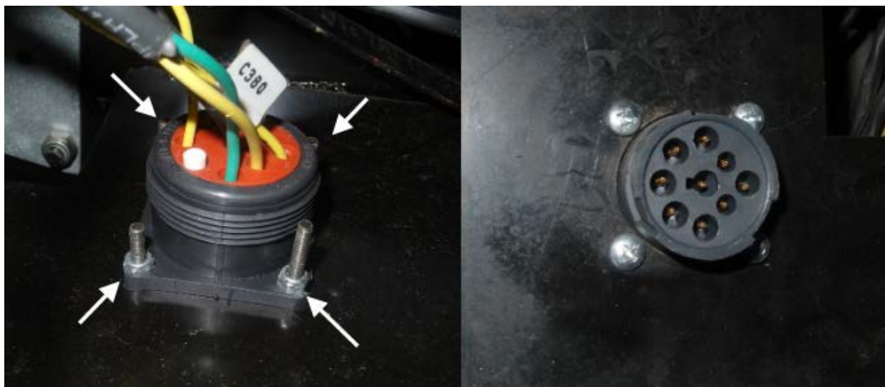
DIAGNOSTIC CONNECTOR SCREWS; BOTH SIDES
