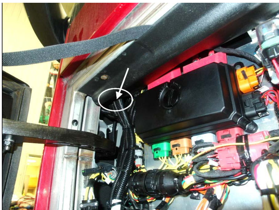
AVOID CONTACT HERE ON H3 VEHICLES
