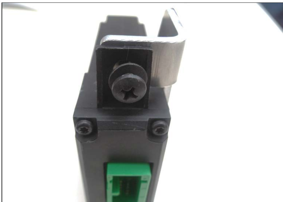
GATEWAY MODULE ON BRACKET – USE FLAT WASHERS
