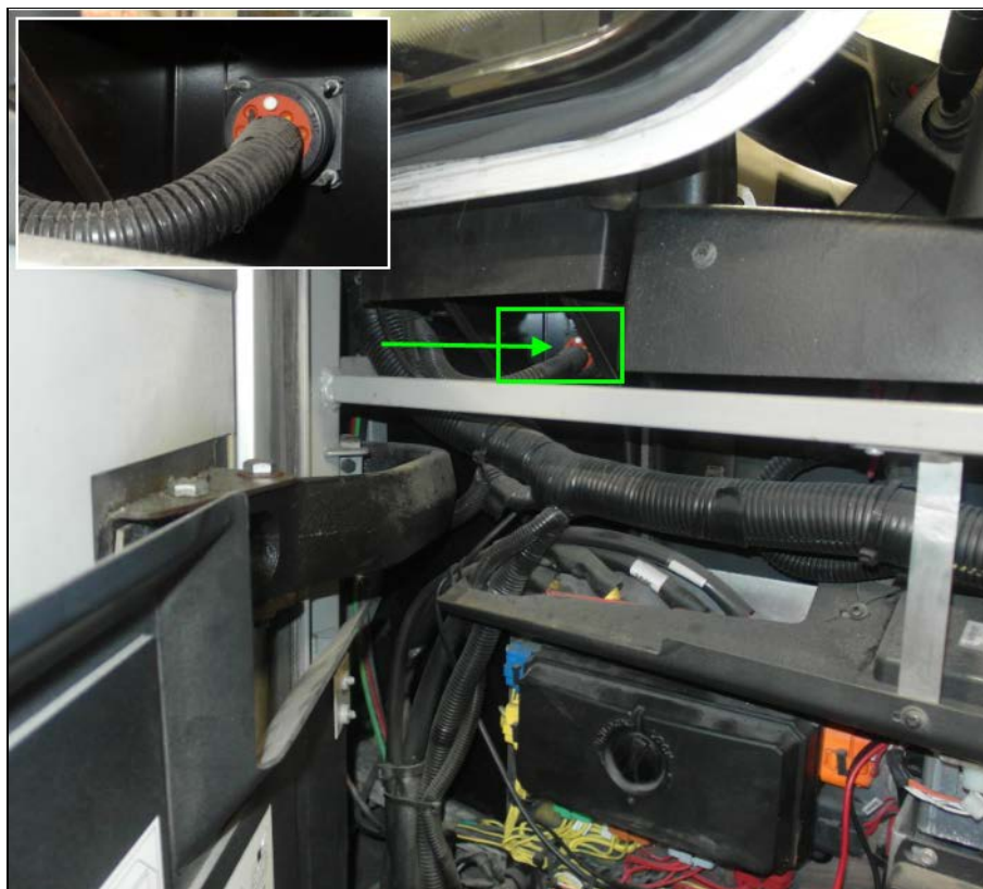
DIAGNOSTIC CONNECTOR POSITION (X3 VEHICLES)
