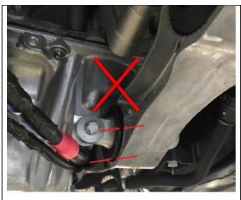
4. Inspect the rubber mount of the engine stabilizer link.
