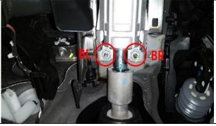
3. Completely release the 2 lower steering adjustment attachment nuts (marked with BR and BL).
