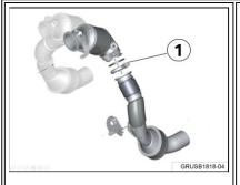
The screw clamps that secure the upper and lower catalytic converters (1) may loosen over time.
